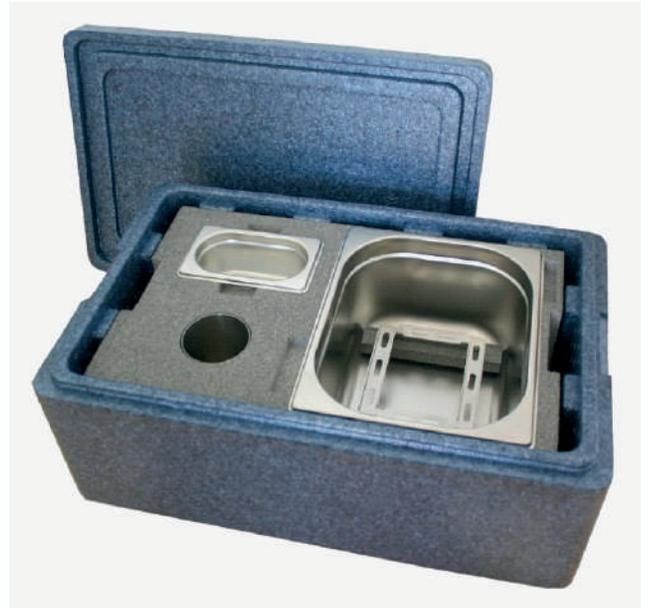
15043/0636 Minitube Freezing unit for 20 straws 0.25 ml and 0.5 ml Each
