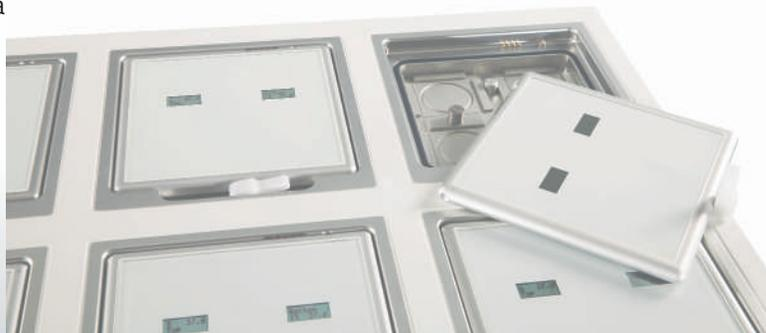
Available 1,2,3 and 4 lid incubator for IVF. Requires Nitrogen and Carbon Dioxide. Internal Filter Inserts specified for standard dishes (35mm) or others as required Removable lids Visual temperature display internally recirculated.
